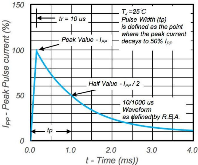
Fig.3 Pulse Waveform
